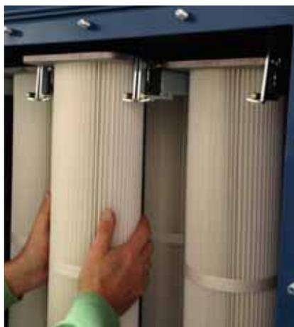
Life-cycle costs of durable industrial goods, to which cartridge filters also belong, are influenced by operating and follow-up costs. This also includes working time for installation and change of filter cartridges. But filter cartridges – as well as with every other filter unit – have to be changed in regular intervals. Compared to common fastening mechanisms, Infastaub has significantly simplified this system.
