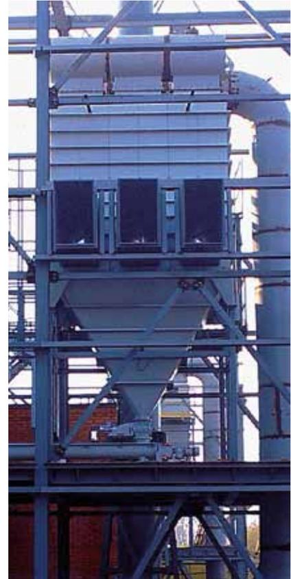
coal dust is present constantly in an explosive dust/air mixture. ATEX zone 22 was identified for the clean gas side and around the filters. As explosion protection strategy constructive explosion design was determined, i.e. all aggregates are made for pressure shock resistant construction with pressure relief via rupture discs. The additional necessary explosion decoupling prevents spreading out a possible explosion into connected aggregates.
