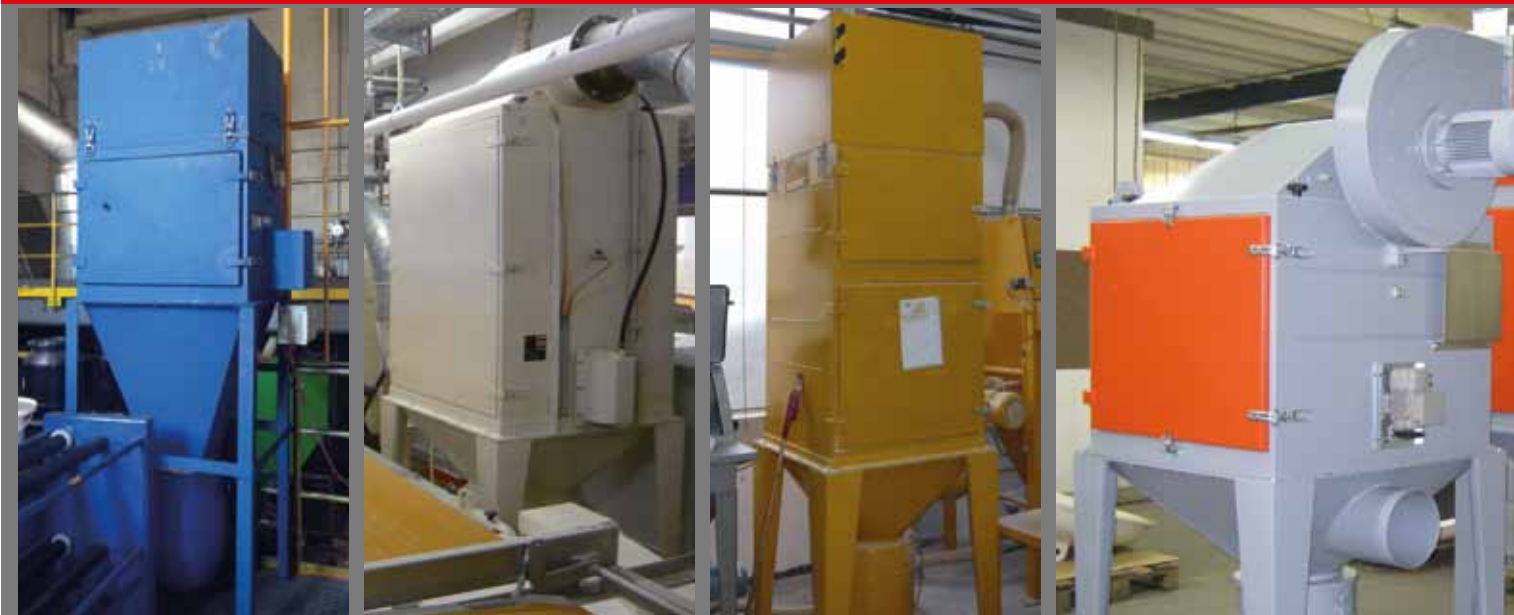
Pocket filter INFA-MAT AM: compact dedusting unit or venting
