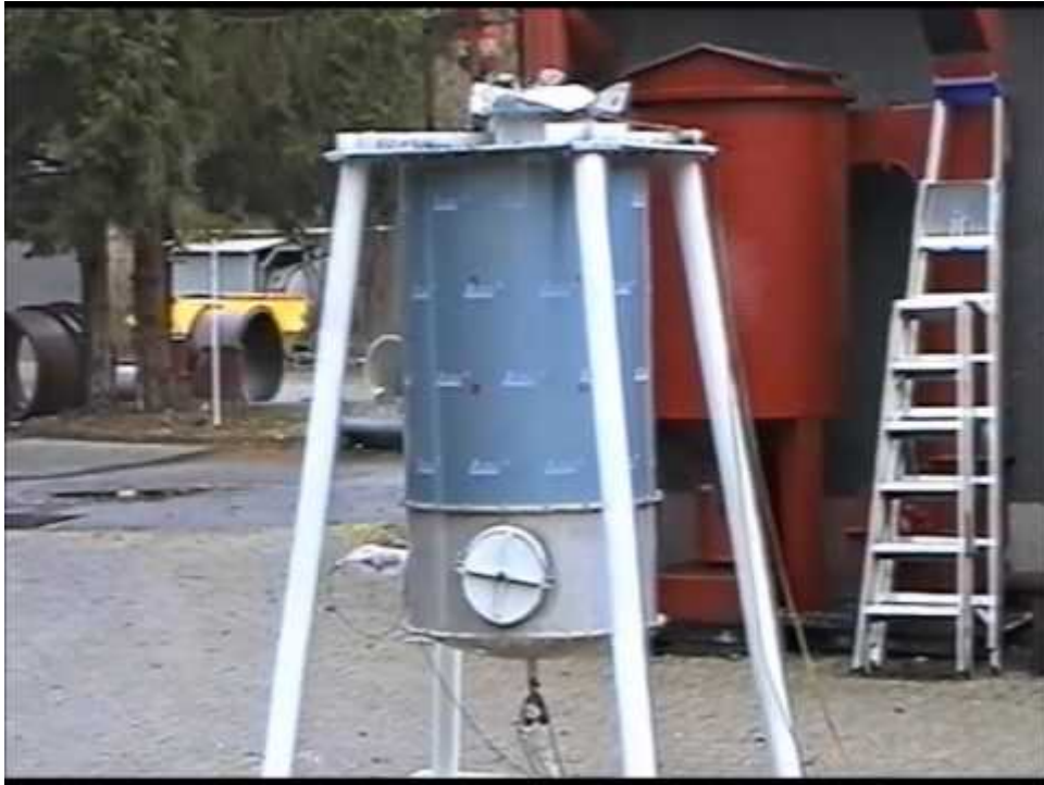
Explosion trials of a cartridge filter INFA-VARIO-JET type AJV to prove pressure shock resistance.
